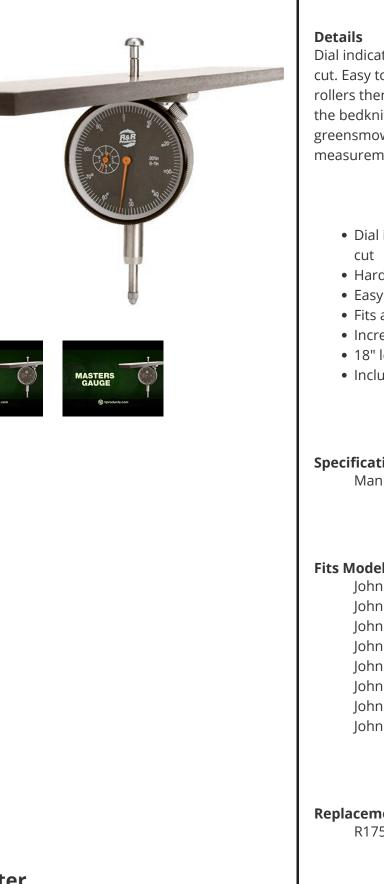
Dial indicator accurately measures desired height of cut. Easy to use. Place the bar on front and rear rollers then push the measuring rod until it touches the bedknife edge. Hard anodized aluminum. Fits all greensmowers. Easy to read dial indicator. Displays measurements in .001" increments. 18" length.
